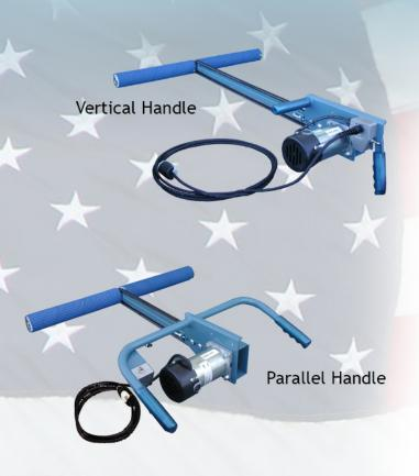
The **Wall Scrubbers** have been designed for removing excess sprayed materials from wall studs, allowing for easy installation of drywall sheathing. The T-frame design allows the contractor to remove excess material from corners with both sides of the rollers. A totally enclosed motor ensures long brush and motor life. The V-belt driven rollers, along with adjustable tensioning feature, provide a light, smooth, positive grip system.
