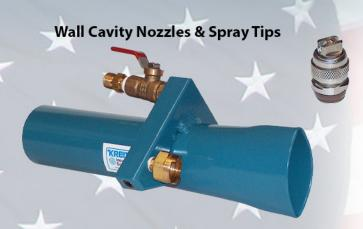
The wall cavity nozzle has a wide oval discharge throat allowing for the maximum flow of coarse, wet, recycled fibers without plugging. Rigid attachment of the spray tip body to internally machined head eliminates misalignment and nuisance pressure tubing leaks caused by frequent accidental impacts. The turn-lock tips offer quick change features.
