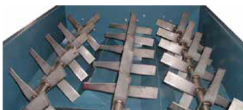
Multiple Agitators Designed for Constant Material Flow
