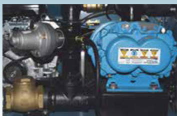
Positive Displacement Blower w/220 CFM @ 5PSI (Electric)
