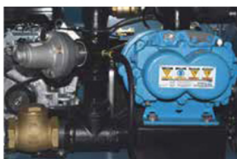
Positive Displacement Blower w/150 CFM @ 6PSI
