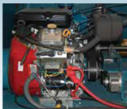
18hp Briggs & Stratton V-Twin Engine w/positive pressure lubrication system.
