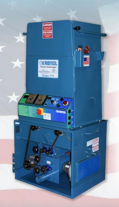
The 575SHA will out perform and outlast the competition. The 575SHA is an economical machine for the professional contractor. Capable of blowing all major brands of cellulose and fiberglass to the manufacturer's specifications, with an additional shredder/agitator to ensure material conditioning and coverage.
