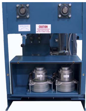
Double Blower System With improved Direct Air Flow 12.5 Amp/3-Stage (120volt)
