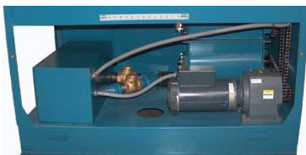
2 HP Direct Drive Motor/Reducer for Increased Torque/ Reduced Amperage
